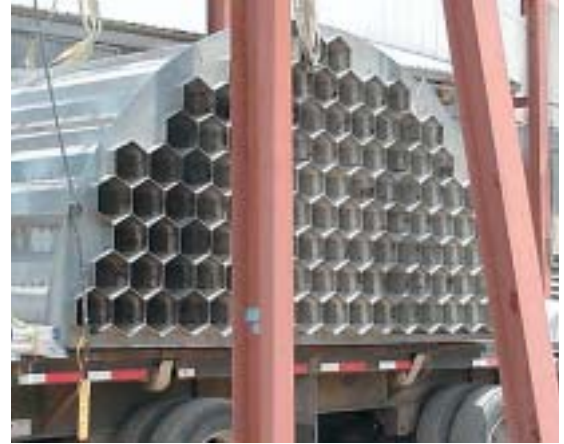
Tube bundle staged for shipment
