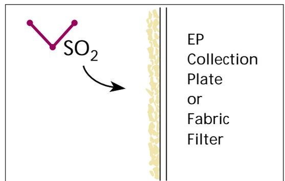
Fig. 4—Residual fine Ca(OH)<sub>2</sub> is captured in the dust collector and continues to react with remaining SO<sub>2</sub> gas.
