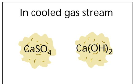
Fig. 3—"Dried" CaSO<sub>4</sub> salt and residual Ca(OH)<sub>2</sub> left over after H<sub>2</sub>O evaporates in GCT.
