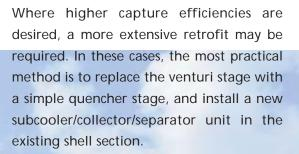
The retrofit is comprised of fieldmodification of the primary quenching or cooling stage, with the rest of the equipment typically shipped in one section for ease of on-site installation. The new section is shipped with a solid diaphragm plate carrying multiple, parallel collector tubes, mounting ports for nozzle lances and a pre-installed separator stage for field installation in the existing shell section.
