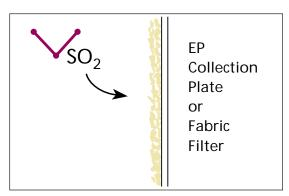
Fig. 4—Residual fine  $Ca(OH)_2$  is captured in the dust collector and continues to react with remaining  $SO_2$  gas.
