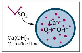
Fig. 1—SO<sub>2</sub> gas is absorbed into water droplets. Ca(OH)<sub>2</sub> ionizes in the water droplet.
