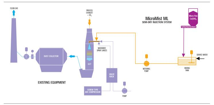
MicroMist ML Micro-fine Lime Process & Instrumentation Diagram (Typical)
